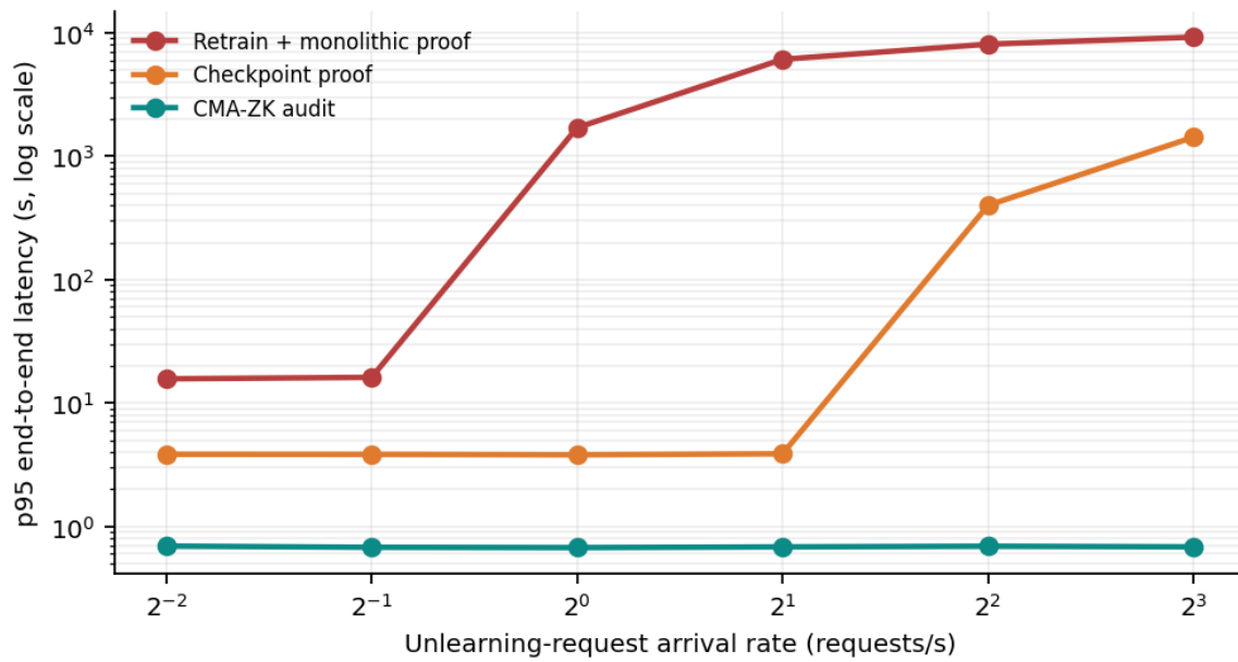
Figure 1. Simulated p95 end-to-end latency across request arrival rates. Both axes use logarithmic scaling. Queue growth occurs after arrival exceeds the modeled service capacity.
